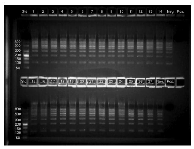
The above results show that there is no degradation of the substrate DNA after incubation with the swabs. The swabs are considered to be DNase-free and PASS.
